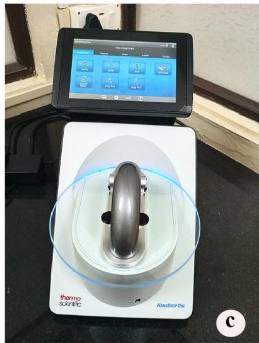
Plate 1. a. PCR thermal cycler- for the amplification of DNA b. Centrifuge- to separate substances of different densities c. Nanodrop - to quantify the amount of DNA d. GelDoc Imaging system- to visualize and capture images of DNA.
