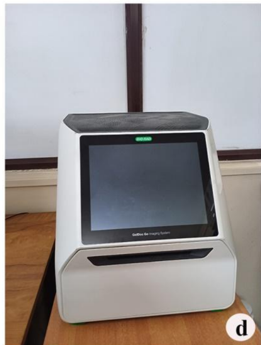
Plate 1. a. PCR thermal cycler- for the amplification of DNA b. Centrifuge- to separate substances of different densities c. Nanodrop - to quantify the amount of DNA d. GelDoc Imaging system- to visualize and capture images of DNA.
