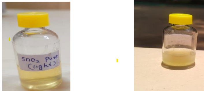
Figure.3.6 Methyl orange solution with SnO 2 NPs after 24 hour and after 48 hour placed under irradiation of direct sunlight
